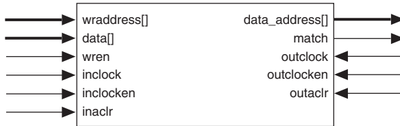
Figure 23. APEX 20KC CAM Block Diagram
