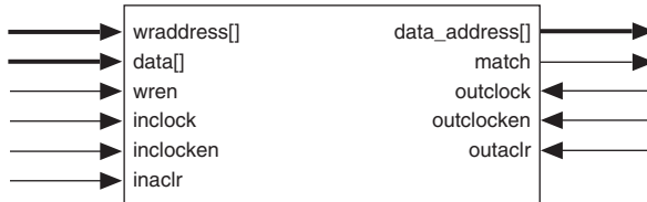
Figure 23. APEX 20KC CAM Block Diagram
