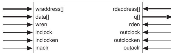
Figure 17. ESB Block Diagram
