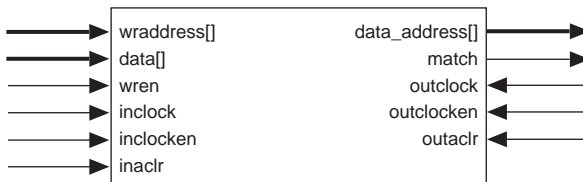
Figure 23. APEX 20KE CAM Block Diagram
