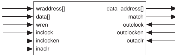
Figure 23. APEX 20KE CAM Block Diagram
