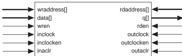
Figure 17. ESB Block Diagram
