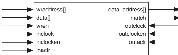
Figure 23. APEX 20KC CAM Block Diagram
