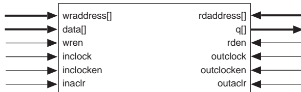
Figure 17. ESB Block Diagram
