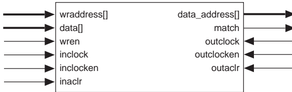
Figure 23. APEX 20KE CAM Block Diagram
