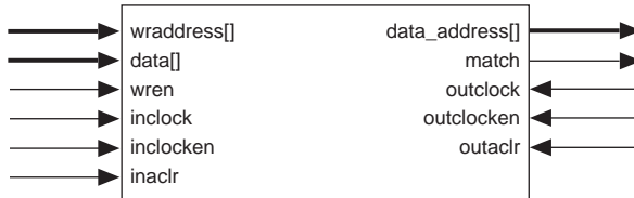
Figure 23. APEX 20KE CAM Block Diagram
