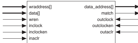
Figure 23. APEX 20KE CAM Block Diagram
