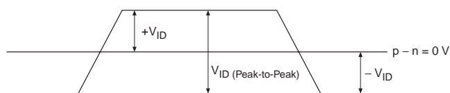
Figure 39. Transmitter Output Waveforms for Differential I/O Standards
