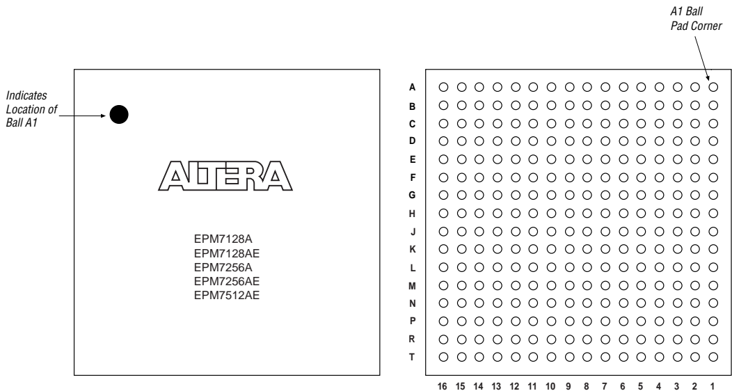
Figure 23. 256-Pin FineLine BGA Package Pin-Out Diagram
