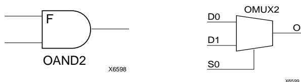
Figure 20: AND & MUX Symbols in XC4000X IOB
