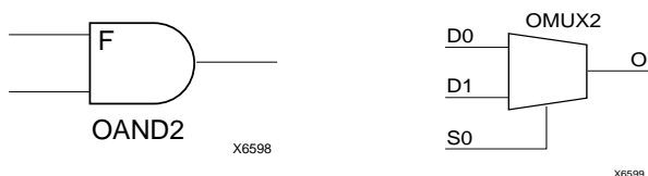
Figure 20: AND & MUX Symbols in XC4000X IOB
