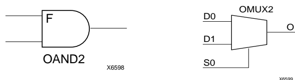
Figure 20: AND & MUX Symbols in XC4000X IOB
