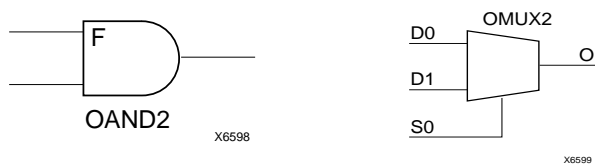
Figure 20: AND & MUX Symbols in XC4000X IOB
