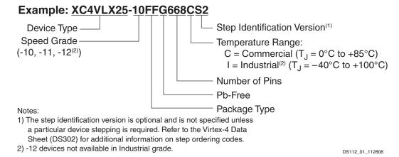
Figure 1: Virtex-4 FPGA Ordering Information
