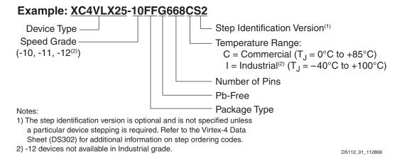
Figure 1: Virtex-4 FPGA Ordering Information
