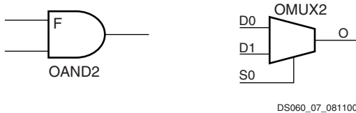
Figure 7: AND and MUX Symbols in Spartan-XL IOB
