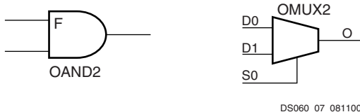
Figure 7: AND and MUX Symbols in Spartan-XL IOB
