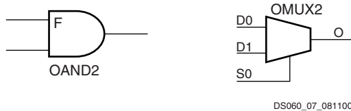
Figure 7: AND and MUX Symbols in Spartan-XL IOB
